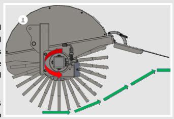
the verge, negating the requirement for a second process of blowing or sweeping the material after weed brushing. A heavy duty guard guides the direction of the material for accurate placement on the verge. 30 Heavy duty hausa brushes remove heavy material from path edges to leave a clean surface.
