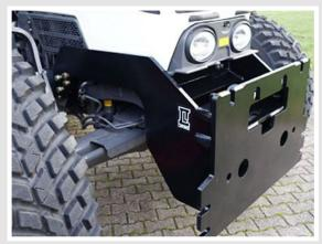
ABR 60 Tele DP - Multiple tractors? Our special bracket and connection system makes it possible to fit the sweeper to a Variety of linkage systems all from the same bracket. This allows it to fit to a tractor front loader, Telescopic loader, front loading shovel hitch and a Tractor 3 point linkage with CAT 1 or CAT 2 link arms.
